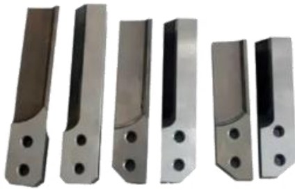
Figure 2. Various Types of KAM Cutters
