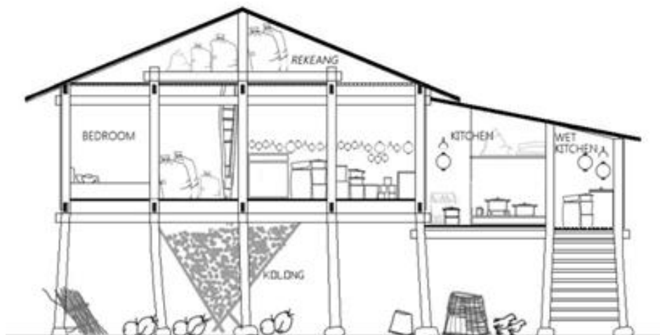
Figure 5: Section of Karampuang domestic house ( bola )
