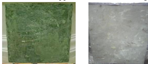
Fig. 13. The color of the material resulting from the melting of plastic waste
