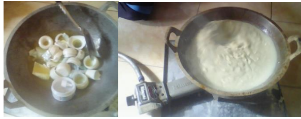
Fig. 3. The melting of plastic waste
