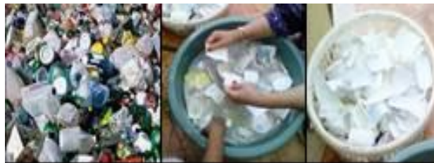
Fig. 1. Plastic waste through a process of washing and drying
