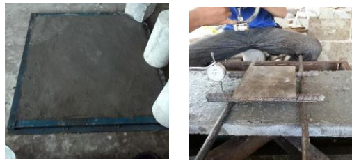
Figure 5. Casting HPFRC plate and Preparing loading test
