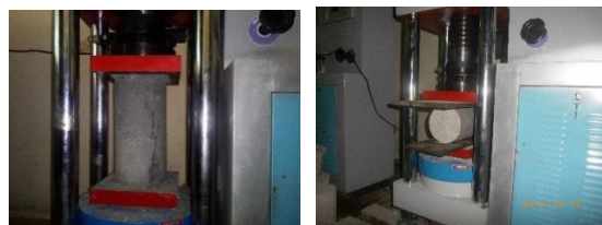
Figure 4. Compressive and splitting test of HPFRC cylinder
