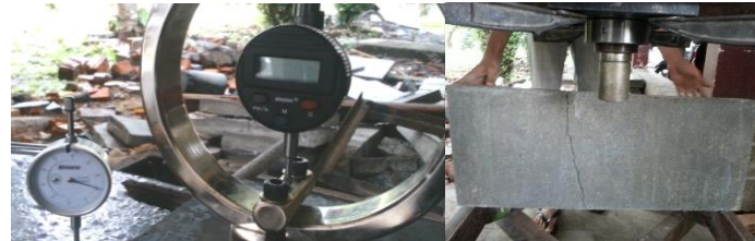
Figure 6. Setting proving ring and dial gauge, bending pattern of HPFRC plate specimens
