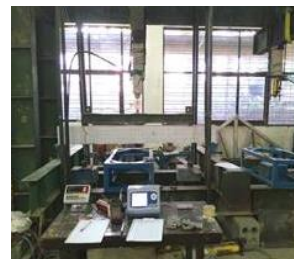
Figure 4. Four-point loading test set up for beam
