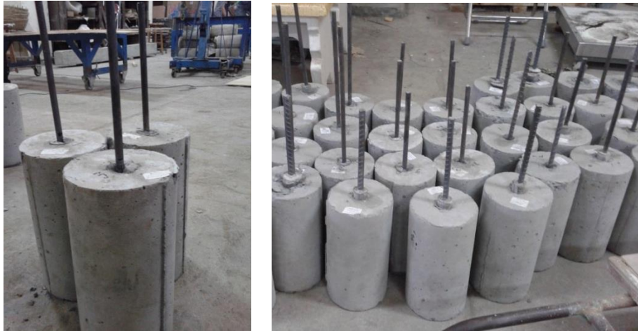
Figure 2. Test specimens of bond pull out
