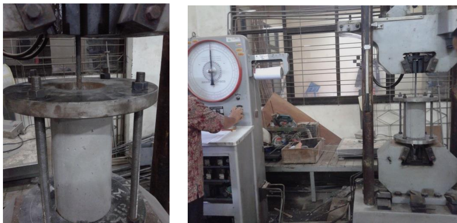
Figure 3. Setting Bond Pull Out Testing
