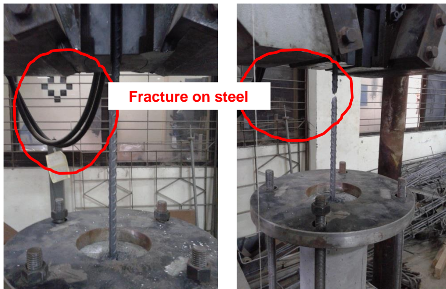
Figure 6. The test results fracture the steel reinforcement
