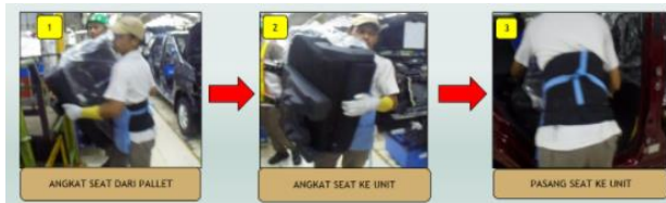
Figure 1. The process of lifting and raft seat work into a motor product
