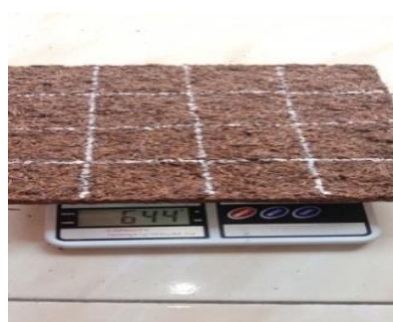
Figure 4. Particleboard weighing 60% adhesive percentage
