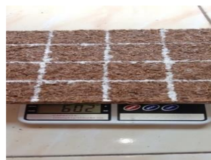
Figure 7. Weighing of particleboard adhesive percentage 75%
