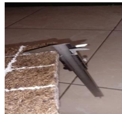
Figure 8. Measuring the thickness of the board Using a caliper on the board 75% percentage
