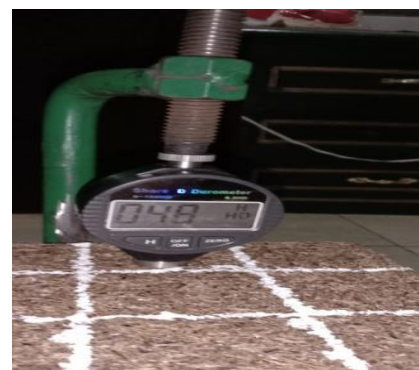
Figure 6. Particleboard test of 75% adhesive percentage with durometer
