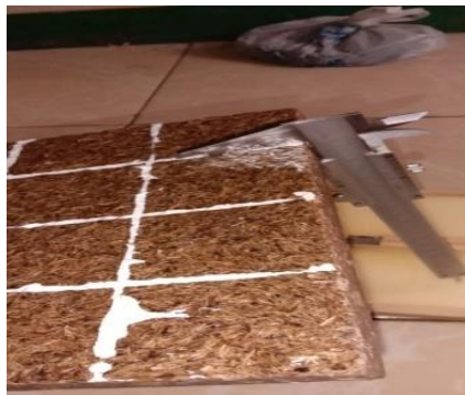
Figure 11. Measuring the thickness of the board using a caliper on the board with a percentage of 90%
