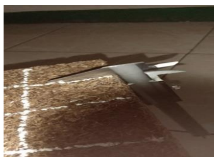
Figure 5. Measuring the thickness of the board Using a caliper on the board percentage 60%
