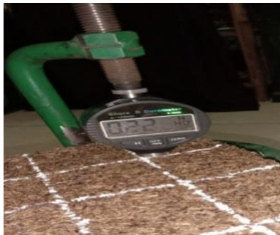
Figure 3. Particleboard test of 60% adhesive percentage with durometer
