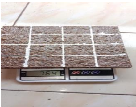
Figure 10. Weighing particleboard adhesive percentage 90%
