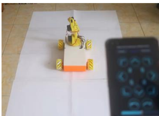
Figure 7. Wheel movement tests on carpet (above) and paper (below) surfaces.
