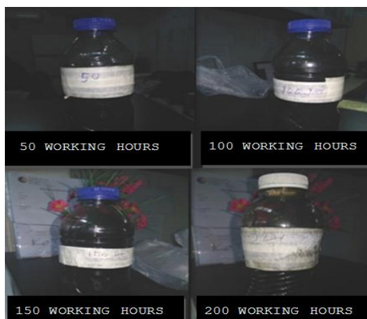
Fig 2. Use of lubricating oil 50,100,150 and 200 hours of engine work
