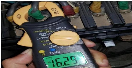
**Fig. 3.** Measurement of electric current and voltage
