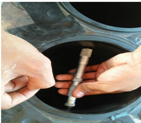
Fig. 6. Measuring cylinder liner
