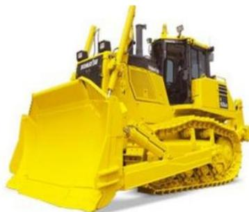
Fig. 1. Bulldozer unit of D375A-6R [1]
