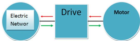
**Fig. 4.** Direction of regenerative drive current
