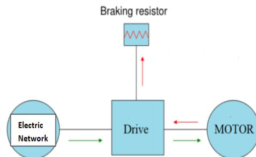
**Fig. 5.** Illustration of non-regenerative drive current direction
