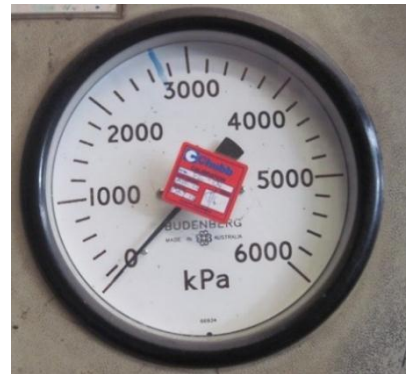
Fig. 5. Pressure gauge 6000 kPa in capacity.
