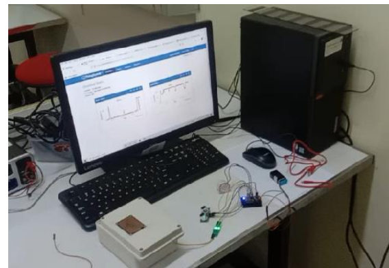
Gambar 2. Sistem monitoring potensi banjir berbasis IoT
