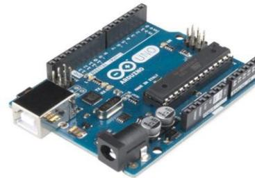
Gambar 2.6 Board Arduino Uno R3
