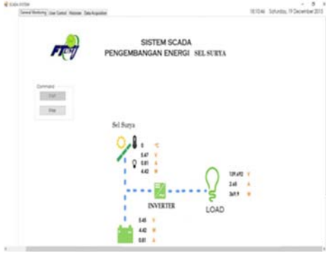
Gambar 4 Interface General Monitoring sistem SCADA
