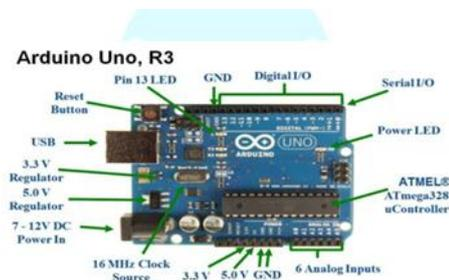
Gambar 2.2 Papan Bord Arduino UNO
