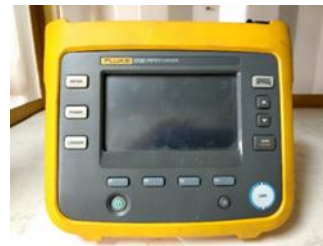
Gambar 7. Power Quality Analyzer
