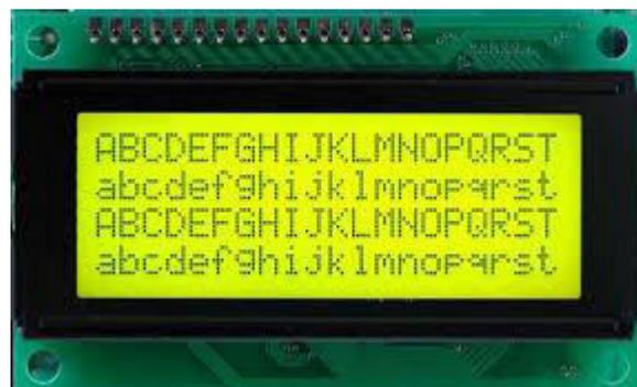
Gambar 2.5 LCD 20x4
