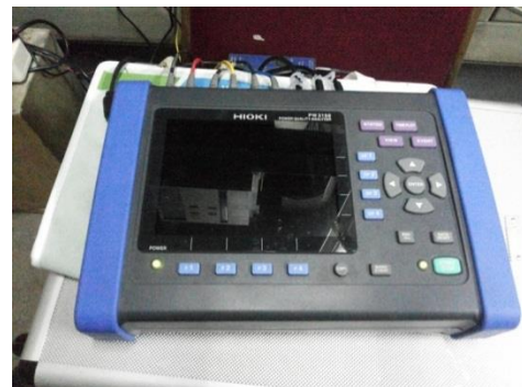
Gambar 3.4 Foto Power Quality Analyzer Hioki PW3198
