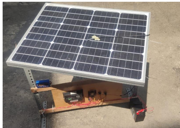
Figure 6: Testing Monitoring of Solar Panel Overheating Detection
