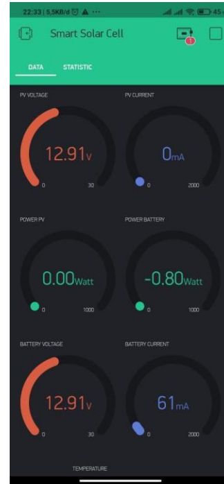
Figure 2: Monitoring of Solar Panel Overheating Detection on the Blynk App
