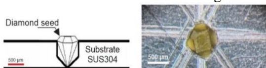
Figure 1. Arrangement of diamond seed and the substrate.
