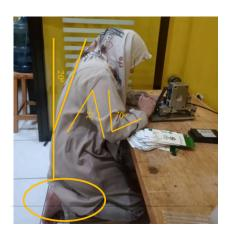
Based on the posture of worker 1 above, there are several angles formed by the worker's body. The angle at the upper arm is 35 degrees. The angle at the lower arm is 70 degrees. The wrist forms an angle of 10 degrees. Based on the following data, the RULA value for group A for worker 1 is 4.
