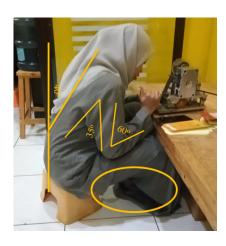
Based on the posture of worker 2 above, there are several angles formed by the worker's body. The angle at the upper arm is 35 degrees. The angle at the lower arm is 70 degrees. The wrist forms an angle of 10 degrees. Based on the following data, the RULA value for group A for worker 2 is 4.
