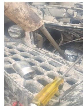
Figure 5: Filter removal using a tommy bar method
