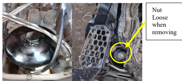
Figure 3: Detached locking nut during filter removal
