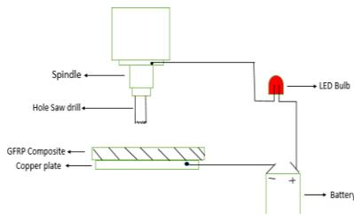
Fig. no. 5. Arrangement for calculating machining time with Hole Saw drill
