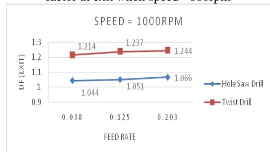
Fig. 16. Comparison between feed rate and Damage factor at exit when speed =1000rpm
