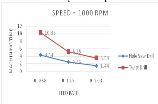
Fig. 10. Comparison between feed rate and machining time when speed =1000rpm
