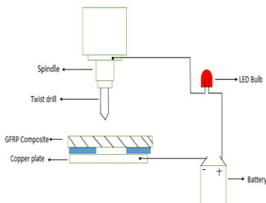
Fig. 6. Arrangement for calculating machining time with Twist drill
