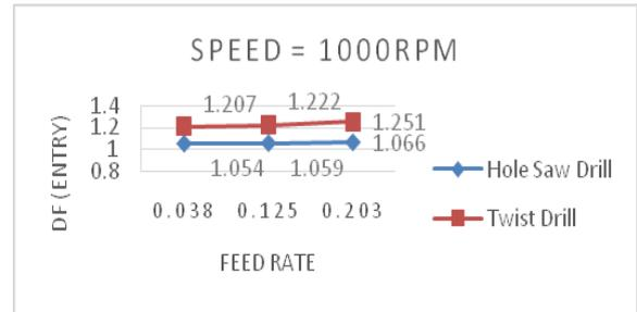
Fig. 13. Comparison between feed rate and Damage factor at entry when speed =1000rpm
