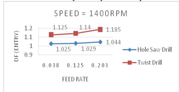
Fig. 14. Comparison between feed rate and Damage factor at entry when speed =1400rpm
