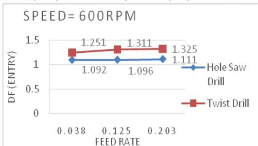
Fig. 12. Comparison between feed rate and Damage factor at entry when speed =600rpm
