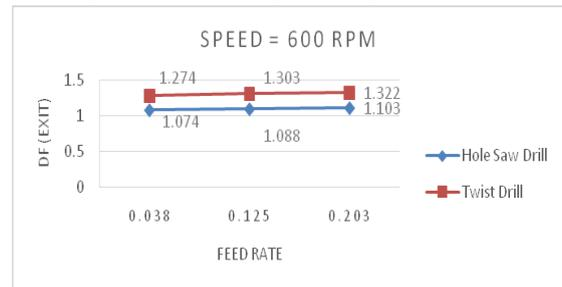
Fig. 15. Comparison between feed rate and Damage factor at exit when speed =600rpm
