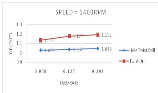
Fig. 17. Comparison between feed rate and Damage factor at exit when speed =1400rpm
