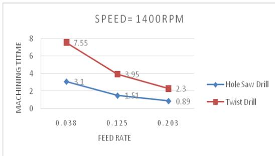
Fig. 11. Comparison between feed rate and machining time when speed =1400rpm
