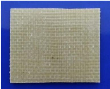
Fig 1. Prepared GFRP Sample
