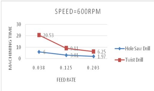
Fig. 9. Comparison between feed rate and machining time when speed =600rpm
