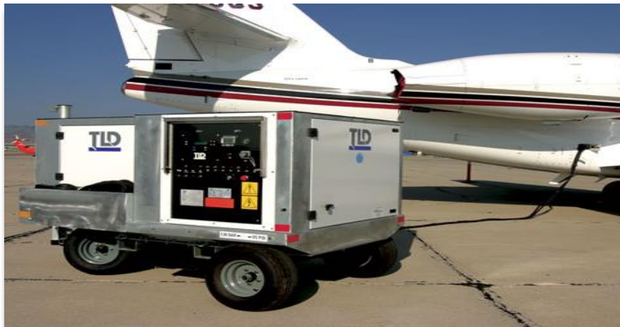
Picture 2. GSE Motorized ( Ground Power Unit). Used for electrical power for aircraft
