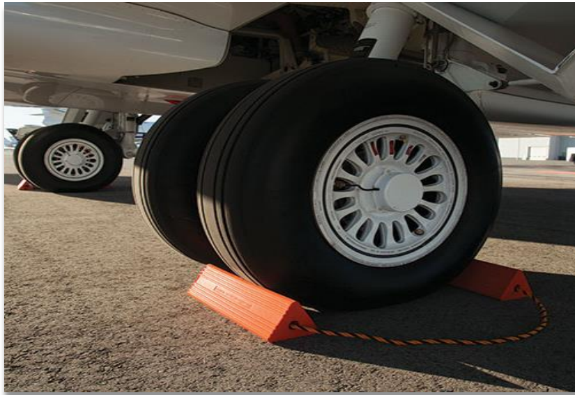
Picture 1. GSE Non Motorized (Wheel Chock) Used to withstand aircraft tires from high winds.
