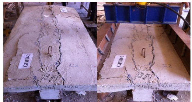
Figure 13. Cracks pattern of specimen GIID-2
