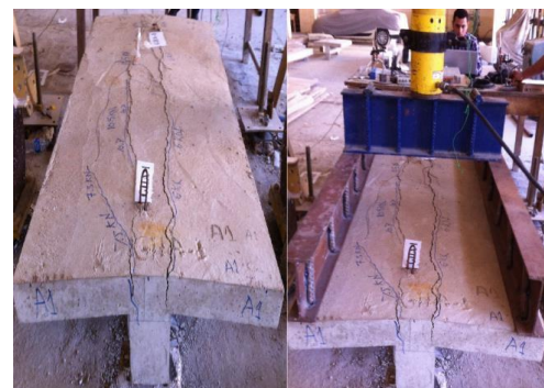
Figure 10. Cracks pattern of specimen GIIA-1
