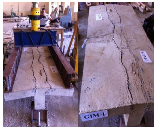
Figure 6. Cracks pattern of specimen GIM-1
