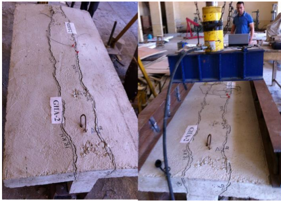
Figure 11. Cracks pattern of specimen GIIA-2
