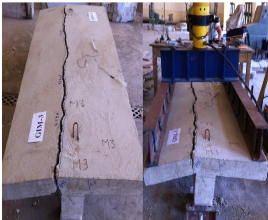
Figure 8. Cracks pattern of specimen GIM-3
