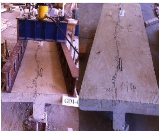
Figure 9. Cracks pattern of specimen GIM-4
