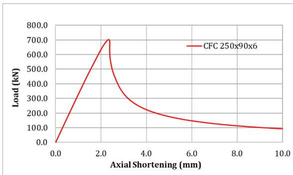
Figure 8. Axial shortening behavior of 250 x 90 x 6 section.
