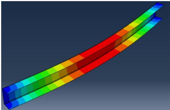
Figure 2. Buckling shape of the first eigenmode of 125 x 64 x 4 section.
