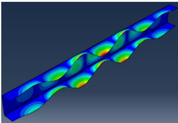
Figure 3. Buckling shape of the first eigenmode of 150 x 75 x 5 section.
