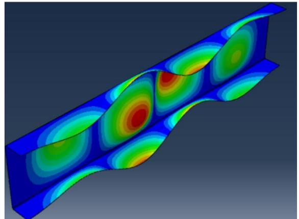
Figure 6. Buckling shape of the first eigenmode of 300 x 90 x 6 section.
