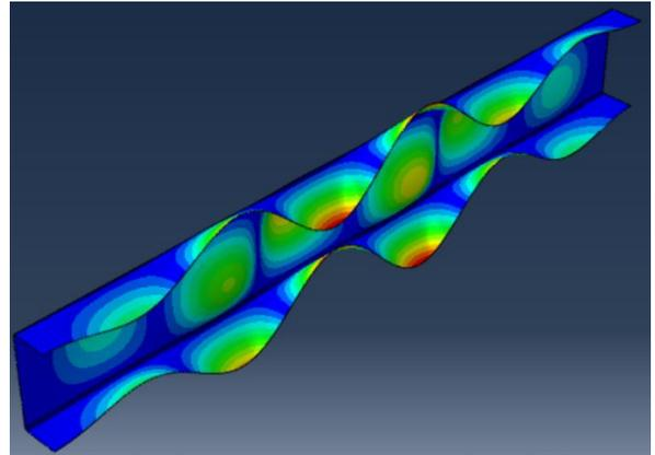
Figure 4. Buckling shape of the first eigenmode of 200 x 75 x 5 section.
