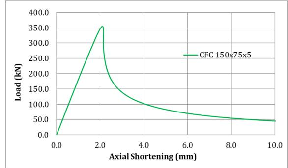
Figure 10. Axial shortening behavior of 150 x 75 x 5 section.
