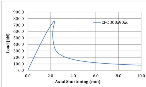
Figure 7. Axial shortening behavior of 300 x 90 x 6 section.
