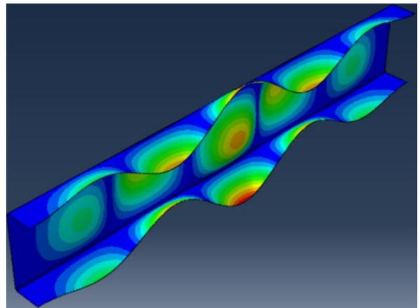
Figure 5. Buckling shape of the first eigenmode of 250 x 90 x 6 section.
