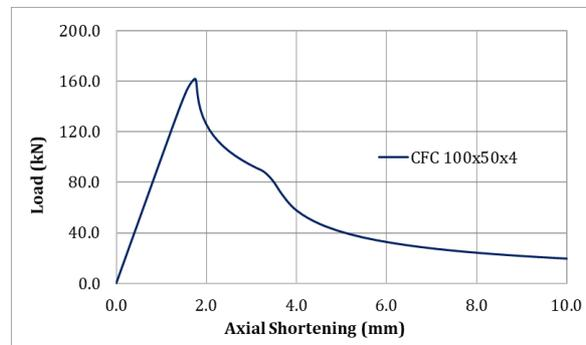
Figure 12. Axial shortening behavior of 100 x 50 x 4 section.
