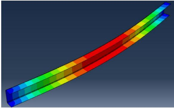
Figure 1. Buckling shape of the first eigenmode of 100 x 50 x 4 section.
