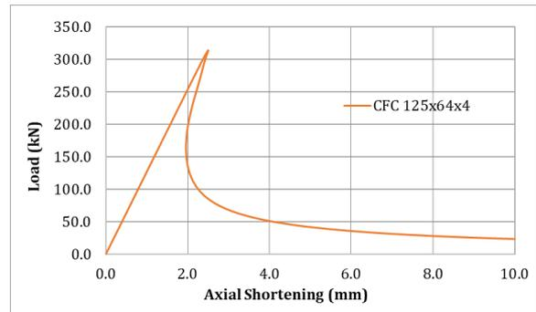
Figure 11. Axial shortening behavior of 125 x 64 x 4 section.
