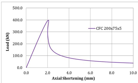
Figure 9. Axial shortening behavior of 200 x 75 x 5 section.
