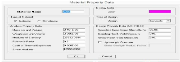
Figure 4.1 Input Material Structure
