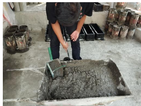
Picture 2. Casting Concrete Mix
