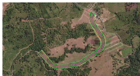
Figure 9. Road Design Geolocation Results (source: Autodesk Civil 3D)
