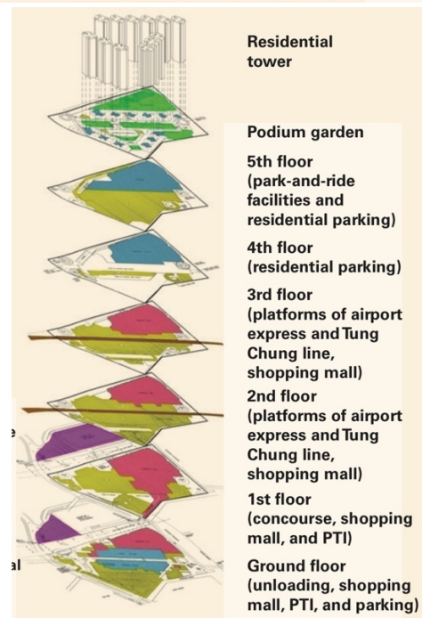
Figure 1: The Maritime Square residential-retail project developed by the Mass Transit Railway of Hong Kong SAR, China
