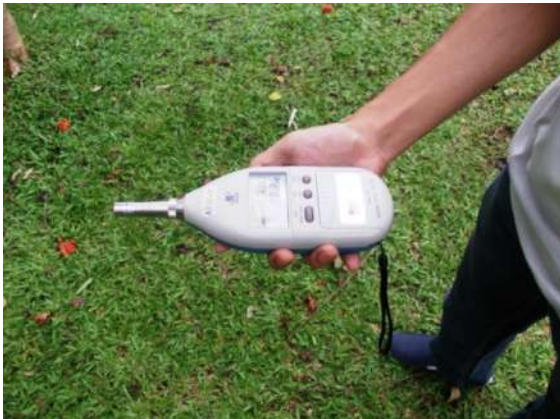
Figure 5 Tool to measure noise level
