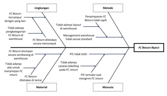
Gambar 3. Diagram fishbone FC retun reject
