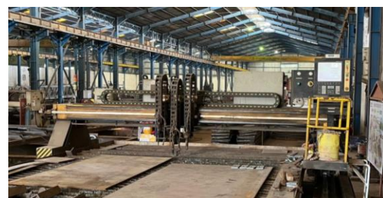
Gambar 4. CNC Flame Cutting Machine Hugong Type GSI1-4500GD
