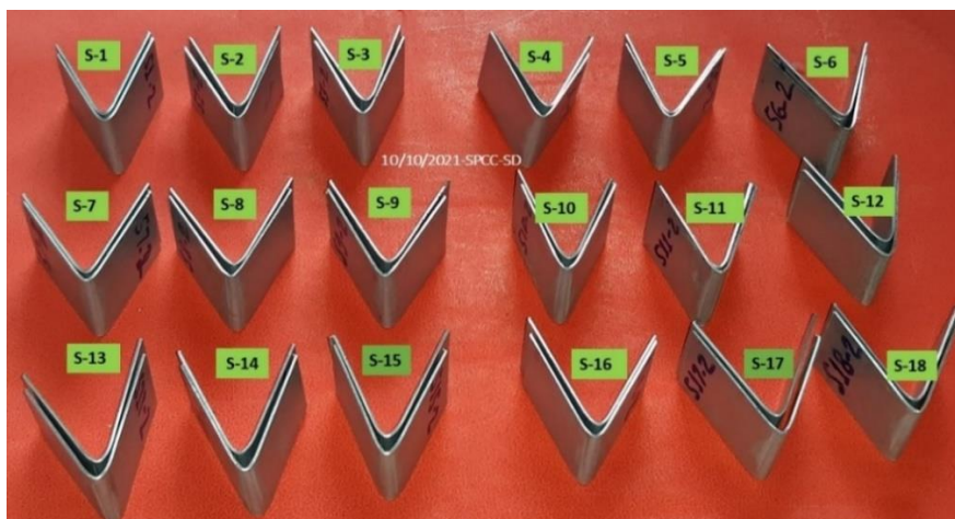
Gambar 4. Sample uji bending sebanyak 18 sample x 2 unit
