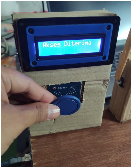
Figure 14. Scanning RFID tags on RFID reader
