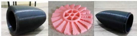
Gambar 4. Hasil 3D-printing ( Duct, fan, motor cone )
