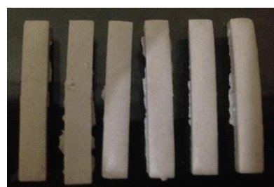
Figure 7. Geopolymer composite sample after heated in the oven at 80°C for 20 hours
