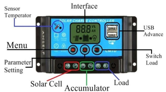
Gambar 3. Fungsi Charger control
