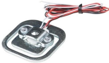
Gambar 3. Sensor Loadcell (Sumber: https://www.lazada.co.id )
