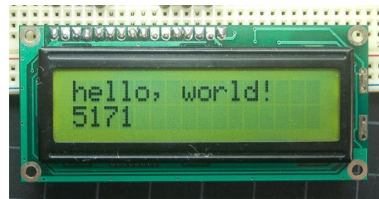
Gambar 2. Liquid Cristal Display 16x2 (Sumber: https://www.arduino.cc )
