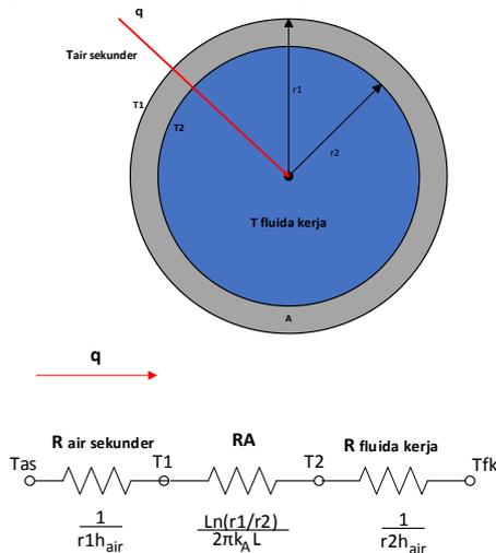
**Figure 4.** One-dimensional thermal flow through a cylindrical cross-section and its electrical analogy
