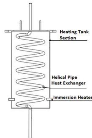
**Figure 3.** Heating Tank Section with Helical Pipe Heat Exchanger.
