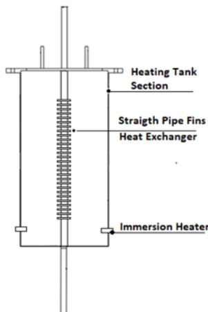
**Figure 2.** Heating Tank Section with Straight Pipe Fins Heat Exchanger.
