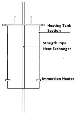
**Figure 1.** Heating Tank Section with Straight Pipe Heat Exchanger.
