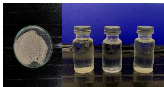
Figure 2. Impregnated Bleaching Earth (left) and Solketal Mixture Before Purification (right)
