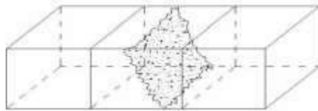
Figure 1. Area 1/3 of the distance of the center placement point (SNI 4431-2011, 2011) the Bending Strength of concrete is calculated according to the following equation:
