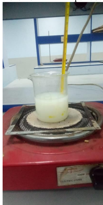
Figure 2. Testing Point Boiling Coolant
