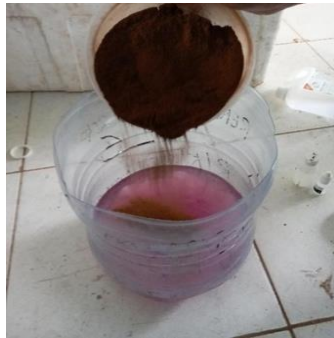
Figure 8. Mixing Ketapang leaves with resin (Source : Serang Engine Workshop)
