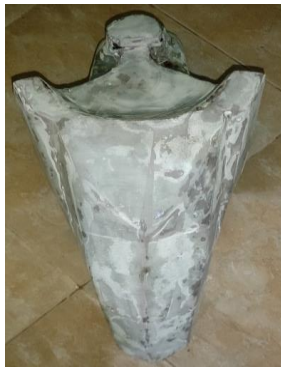
Figure 4. Fenders made with the hand lay up method
