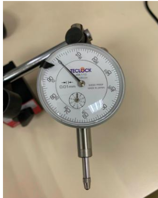
Figure 11. Dial indicator used to measure the repeatability of the robot arm
